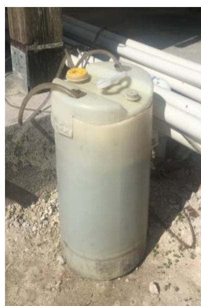
Figure 6: 15 gallon plastic mineralization vessel
