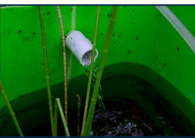
Image 3: Clean water flowing through one of the three treatment systems into a jug of sedge grass.
