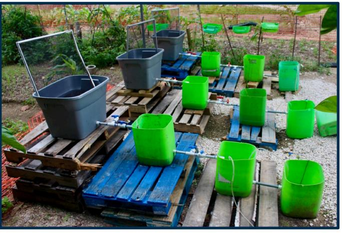
Image 1: Current prototype of the treatment systems built and constructed with 85% recycled material found at the Island School.
