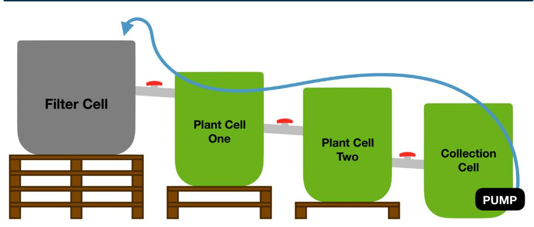
Figure 1: A graphic representation of the initial prototype design, showcasing the four cell system.
