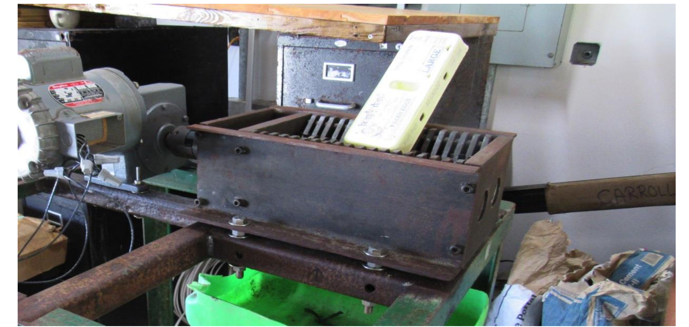
Picture 4: Motorized Shredder.
