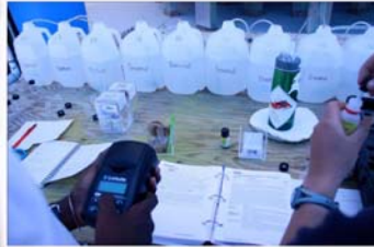
The essential nutrients setup with the one gallon jugs, the testing reactants, and the colorimeter.
